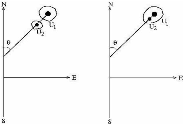
**Fig. 1.** Details of the technique used to measure the shear angle. U1 and U2 are the umbrae of the bipolar sunspot. Angle ‘ $\theta$ ’ gives the orientation of the umbrae in the sunspot on a day. NS is the rotation axis of the Sun.
